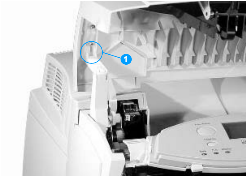
Figure 6-3 Removing and replacing the top cover (1 of 2)
